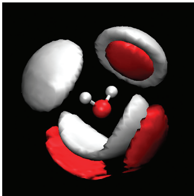
FIGURE 8. Spatial density function of oxygen (red) and hydrogen (white) in the first solvation shell of a (ball-and-stick rendered) water molecule at room temperature, calculated using quantum simulations with the ab initio based polarizable TTM2.1-F water model (see Figure 8 of ref 26 for details). Courtesy of Francesco Paesani and Gregory A. Voth.
